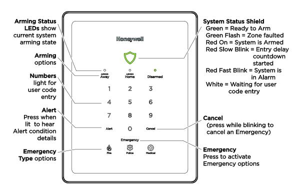
The Gateway Touchpad is designed to operate your basic security features. It also lets you quickly see your system status by which items on the Touchpad are lit.
